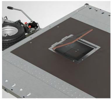
O In-deck storage facility Keep your straps and tools in a convenient place. Latch release catch (not locking).
