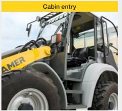
The cabin can be accessed through the large entry area. The undivided vehicle frame also makes it possible to comfortably enter at maximum steering lock. The entry is designed like steps. The grab handles are ideally positioned ergonomically to enable the operator to get in and out easily.
