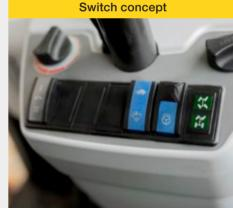
The respective functional group is very quick and easy to identify due to the colour-coded switches. Red = safety, green = hydraulics, blue = travel and grey = electrical system. This ensures the operator a convenient and safe operation without the risk of being confused. The result is increased working efficiency for the operator.
