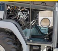
The cleaning flap is located on the right side of the cabin. The flap opens upwards from the bottom using a handle and is fixed by an attenuator. This gives easy access to the cabin air filter and main control equipment. The cabin floor can be cleaned very easily.
