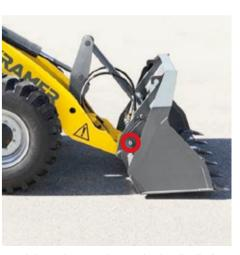
**Hydraulic quick-change system - The Kramer quickhitch system:** approach the attachment, pick up the attachment hydraulically from the operator's seat and lock it using the touch slide on the joystick. The lock cylinder is located outside of the pivot point of the quickhitch plate and is thus not in the contamination area.
