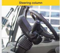
The optional tilt-adjusting steering column can be adjusted to suit the operator's requirements. The steering wheel consists of a high-quality, non-slip material. The steering column also includes a modern dashboard display with automatic blinker reset.
